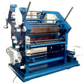
Corrugation Machine E Flute - 42 Inch
